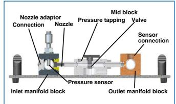
Every outlet manifold block has 3 connections for sensors (1x pressure and 2x temperature). The corresponding measuring values allow to control the critical pressure relation and to see if strong temperature gradients appear. The tightness of the nozzle gallery is assured by O-rings at the relevant joints.
