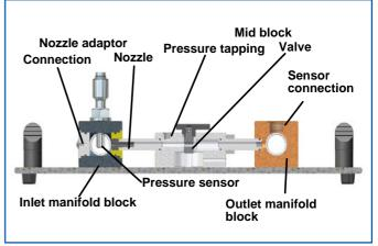
Every outlet manifold block has 3 connections for sensors (1x pressure and 2x temperature). The corresponding measuring values allow to control the critical pressure relation and to see if strong temperature gradients appear. The tightness of the nozzle gallery is assured by O-rings at the relevant joints.
