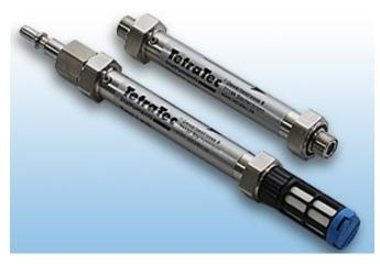
Test leaks are used to simulate leaks when adjusting or monitoring leak testing equipment or as monitoring and adjusting gauges for flow rate measuring devices. They are used in place of the device under test or in parallel to an impermeable device under test.
