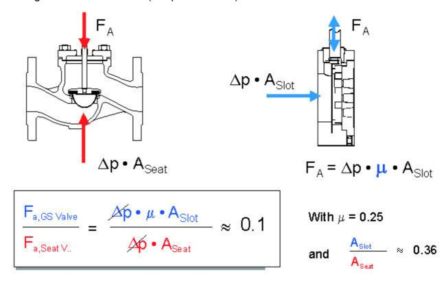
The result is that 10 times less force is required to modulate a sliding gate valve than a single seat globe valve. Furthermore the pressure of the process medium against the moving disc assists the tight seal across the valve.
