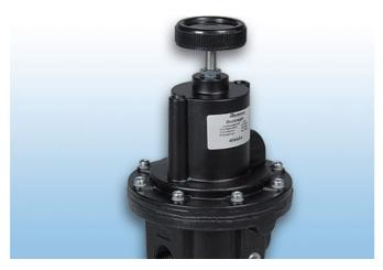
The M4000A pneumatic precision regulator is a direct acting proportional regulator for overpressure with control ranges of 0,035 to 17 bar and flow ranges of 4200 NI/min at 7 bar pirmary pressure.
