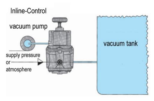
Advantageous connection of the vacuum regulator, if the tank should be filled with overpressure in one case and should be evacuated in the other case. The supply pressure can be opened alternatively to atmosphere.
