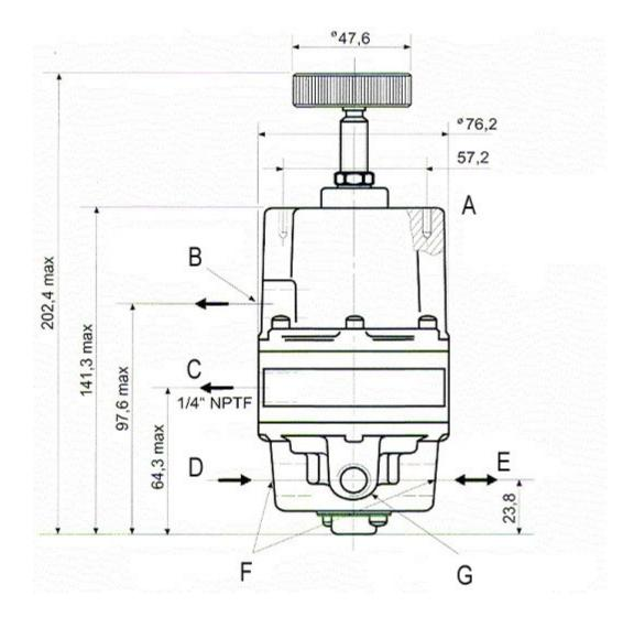
A Mounting threads for mounting brackets
