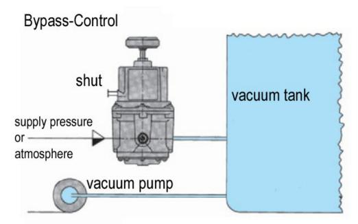
Advantageous connection of the vacuum regulator, if the vacuum tank should be evacuated and controlled very quickly. In this case the vacuum pump operates directly to the vacuum tank and is not throttled through the regulator.
