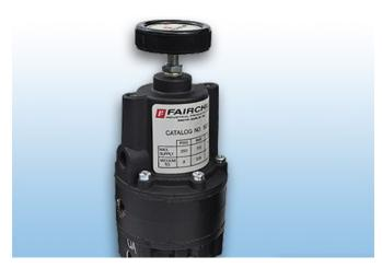
The M16 precision pressure regulator is a direct acting proportional regulator for vacuum and overpressure with regulation range limits from -0,9 bar and +0,15 up to +10,0 bar.
