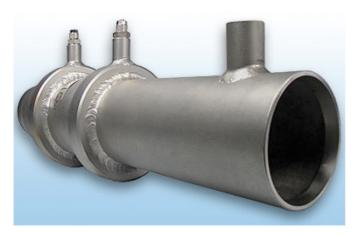
H800 venturi tubes are used for flow rate measurement of aggressive and non-aggressive gases, steams and fluids, especially if low pressure loss is indicated.
