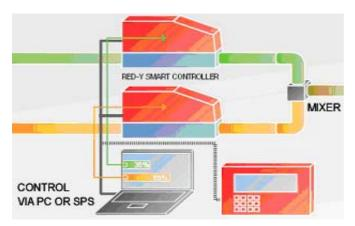
The Process Control Units PCU-10 completes the mass flow meters of the Smart Serie GSx. The unit is useful for visualisation and controlling of the mass flow meters and controllers of the smart series and expands these devices by additional functions.
