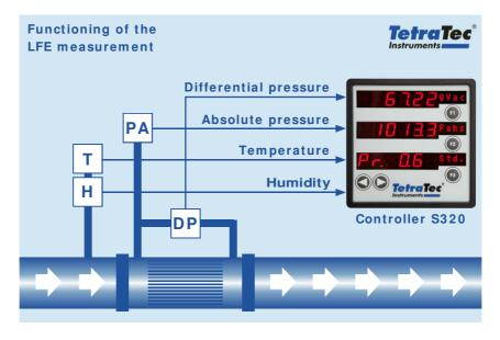
According the Hagen-Poiseuille law the actual volume flow through straight pipes at laminar flow conditions with liquids and gases creates a linear proportional pressure drop  $\Delta p$  dependent to the viscosity  $\eta$  of the flowing media.
