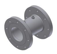
Stainless steel body with integrated stainless steel matrix. Differential pressure connections are 1/4" NPTF, Process connections are flanges acc. ANSI 150 lbs.
