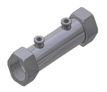
Stainless steel body with integrated stainless steel matrix. Differential pressure connections are 1/4" NPTF, Process connections are threads with NPTF. Differential pressure at nominal flow: 0 - 20 mbar, Operation limits: 0 - 70°C / 0,4 - 10 bar abs
