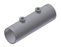
Stainless steel body with integrated stainless steel matrix. Differential pressure connections are 1/4" NPTF, Process connections are plunt tube ends. Differential pressure at nominal flow: 0 - 20 mbar, Operation limits: 0 - 70°C / 0,4 - 6 bar abs
