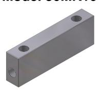
Stainless steel body with integrated stainless steel capillary tubes fixed inside the body with an Epoxy filling. Process and differential pressure connections are threads with 1/4" NPTF Differential pressure at nominal flow: 0 - 20 mbar, Operation limits: 0 - 70°C / 0,4 - 10 bar abs
