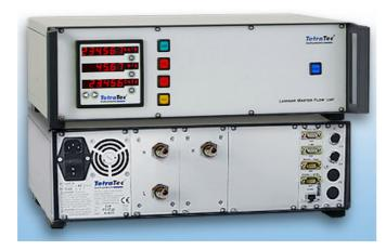
The calibration system LMF-KAL evaluats Laminar Flow Elements (LFE), subcritical orifices, nozzles or other pressure drop elements, as well as critical nozzles, which were used for the calibration of air and gas volume and mass flow.
