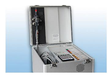
The electronical gas dosing unit LFC injects analysis gas with a pressure controller through a laminar flow element LFE for tightness and function testing into the exhaust gas dilution air of a CVS test bench or shed chamber.
