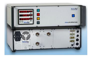
The calibration system CVS-KAL evaluats Laminar Flow Elements (LFE), subcritical SAO nozzles or other pressure drop devices, like Betaflow. These were used for the calibration of the air intake measurement with critical Venturi nozzles in a CVS test bench.
