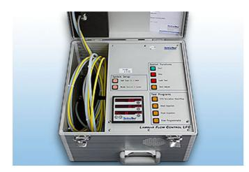
The electronical gas dosing unit CFO-Sx00 injects analysis gas with a pressure controller through a critical flow orifice CFO for tightness and function testing into the exhaust gas dilution air of a CVS test bench.
