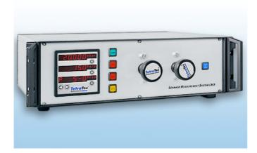
The Leakage Measurement System, LMS in brief, allows leakage measurement with air or gases according to the pressure drop method. An improvement of resolution is achieved by measurement of differential pressure.
