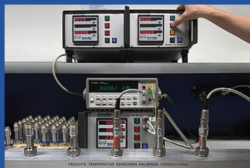
Calibration assembly with a HUMTMP sensor
